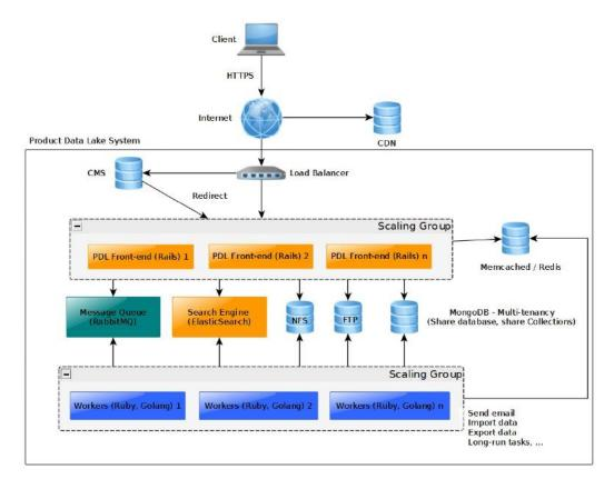
From the outside, end users can access PDL via Internet and be secured with HTTPS protocol (forced) to ensure user privacy. The administrator can use CMS to edit the landing page of PDL, where the public version of PDL is build using LocomotiveCMS. The end users will be redirected to PDL after clicking on Sign in / Sign up. Sign in / sign up can also be called individually in a given language from other websites.
